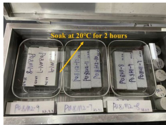
Figure 4 Wet-dry Cycling Test Using a Constant-Temperature Water Bath for Immersion
