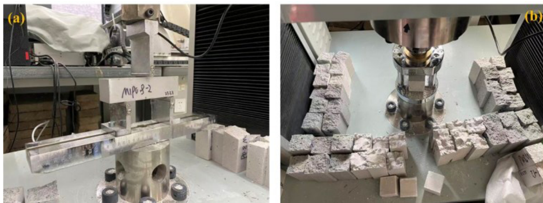
Figure 6 Flexural and Compressive Strength Measurements Conducted with a WDW-300 Electronic Universal Testing Machine: (a) Flexural Strength Test; (b) Compressive Strength Test.
