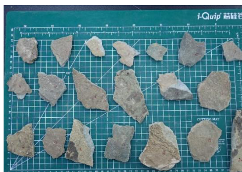
Figure 10 Schematic Diagram of Sheet-Like Detachment Morphology
