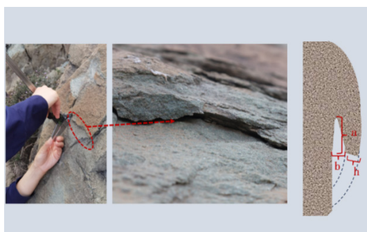
Figure 9 Schematic Diagram of Geometric Parameter Measurements of Splitting
